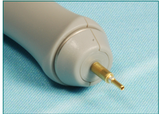
MCP-6 Probe with Coaxial Pin Installed
