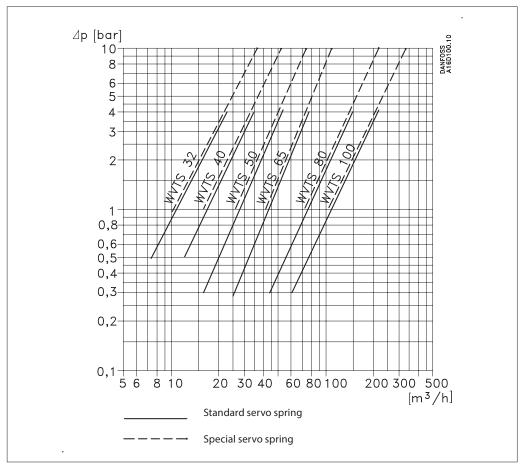
The capacity curves show the capacity (water quantity in  $[m^3/h]$ ) of the individual valve sizes as a function of pressure drop across the valve.
