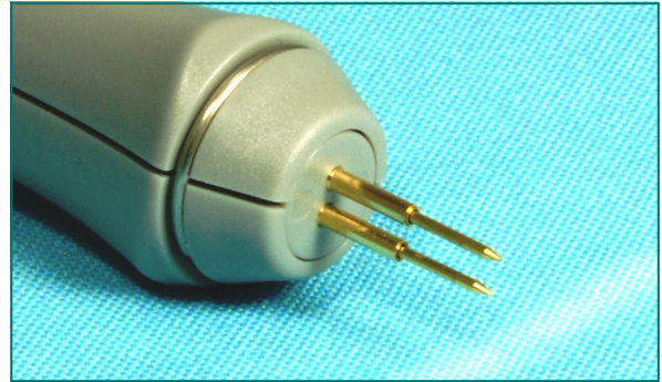
MKP-6 Probe with "B" Style Pin Installed
