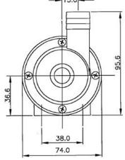
mounting foot fixing holes:M5
