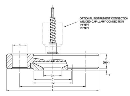
X = Number of Bolt Holes DN = Nominal Pipe Size DM = Effective Diaphragm Diameter CLASS = Flange Rating Per ASME B16.5 All Dimensions in inches unless otherwise noted
