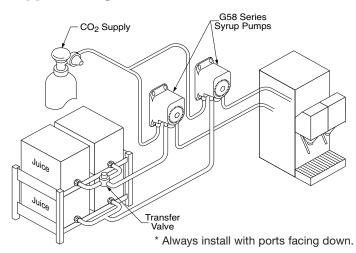
The diagram above shows a "typical Bag-in-Box installation" with a single bag connection and a multiple bag connection with a Flojet Transfer Valve assembly. Flojet Part Nos. 1500-031 and 1500-131 transfer valves recommended for automatic unattended change-over from empty to full bag for all G58 pumps.
