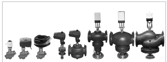
The AB-QM valve equipped with an actuator is a control valve with full authority and an automatic balancing function / flow limitation. Typical applications are: Temperature control with permanent automatic balancing on terminal units (chillers, air-handling units, fan coils, induction units, radiation panels and heat exchangers).
