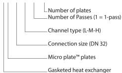
1-pass gasketed heat exchangers type XGM032 (PN 16)
