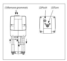
The manual override is applied by rotating the 8 mm Allen key (not supplied) to the required position. Observe the direction of rotation symbol.
