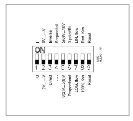
The actuator has a function selection DIP switch under the removable cover. In particular, if SW6 is set to ON, the actuator will perform as 3-point actuator.
