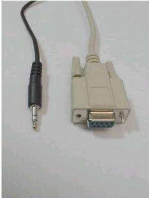
Attaching the Interface Cable TDL-SC Interface Cable for serial port (same concept for DL700)
