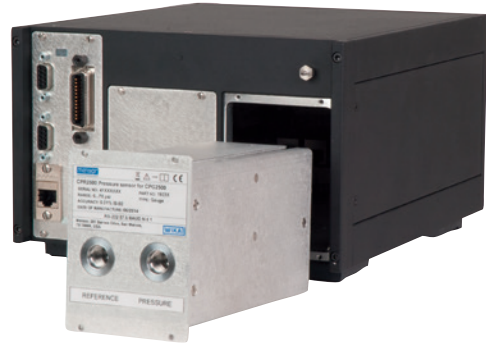
Removable / replaceable reference pressure sensor
